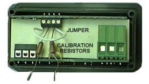
**Step 6:** Install the jumper cable between the loose end of one of the resistors and the fixed end of the other resistor to establish an input value of a single resistor (i.e. 1000 ohms or 100 ohms), as shown.
