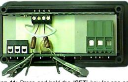
**Step 11**: Press and hold the "**SET**" key for one second. The display will read "**HoLd**". Wait for the display to reset. After it resets, the display should indicate the approximate temperature value for the connected precision resistors (i.e. 511°F or 266°C).
