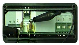
**<u>Step 6</u>**: Carefully restore power to the control, taking precautions not to make contact with any exposed voltage sources.
