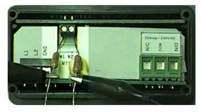
**<u>Step 10</u>**: Press and hold the "**SET**" key for 1 second. The display will read "**HoLd**". WAIT for the display to reset. After resetting, the display should indicate the approximate temperature value for the connected precision resistors (i.e. 511°F or 266°C).
