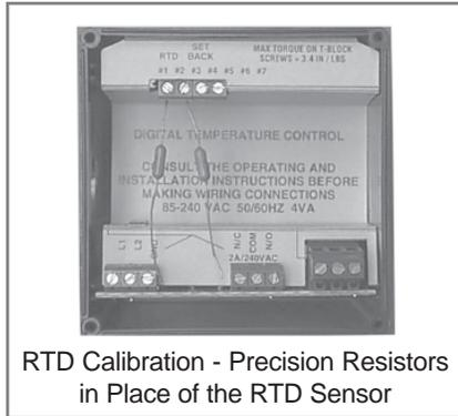
RTD Calibration - Precision Resistors in Place of the RTD Sensor
