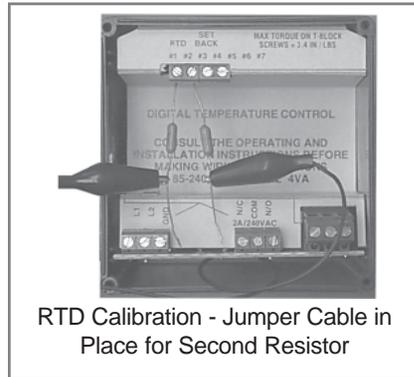
RTD Calibration - Jumper Cable in Place for Second Resistor
