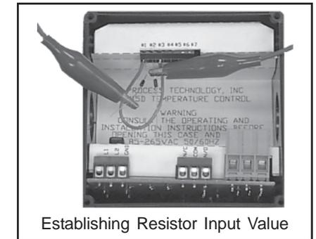
Establishing Resistor Input Value
