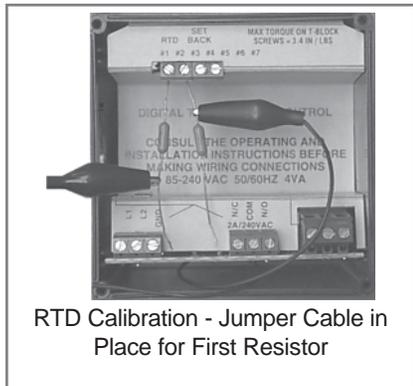
RTD Calibration - Jumper Cable in Place for First Resistor
