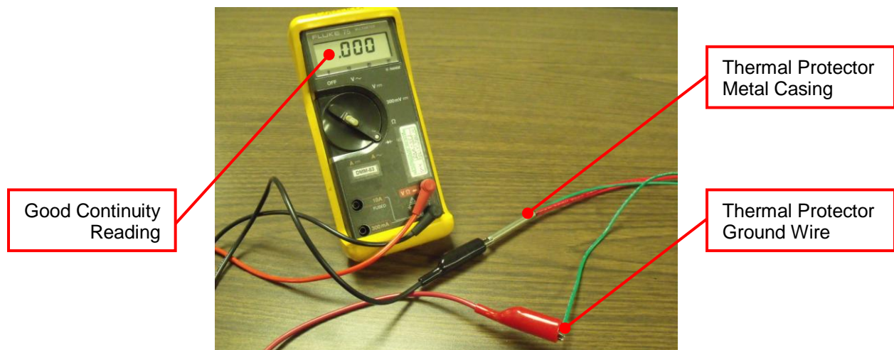
Figure 2: Continuity Check Using Multimeter
